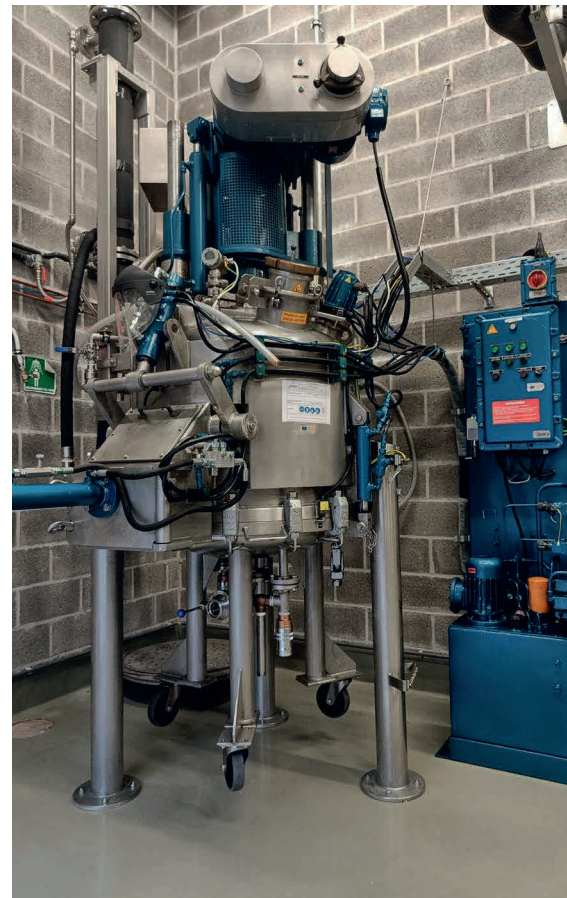
Pilot scale extraction: prototype production to confirm the extraction protocols established at lab scale.
